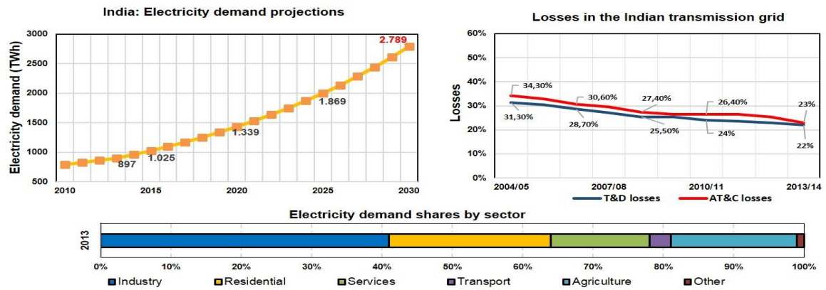
Figure 8.3. Electrical demand increase, grid losses, and the demand shares by sector in India
