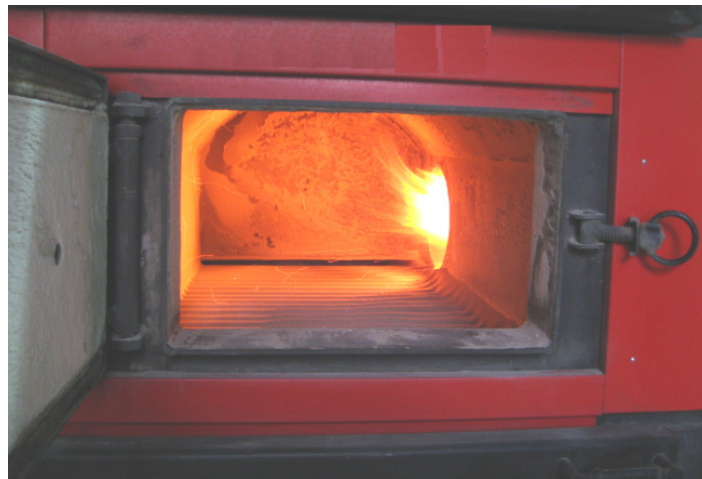
Figure 2: Industrial wood chips pre-furnace/gasifier. Typical application for hot water heating systems [Error! Reference source not found.]
